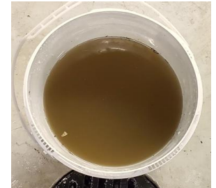
Particulate removed from Condenser water after 24-hours with ElectroCell
